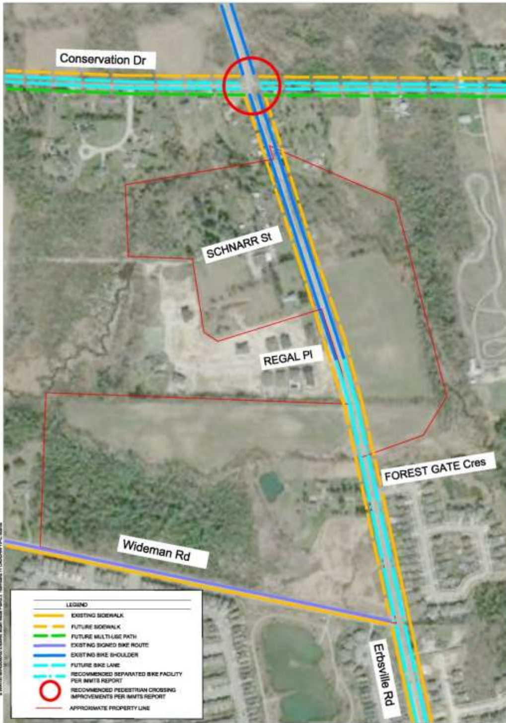
Figure 5-3 Future Active Transportation Network Erbsville South Block Plan Transportation Study 18M-02095-PIC Board_20190328.dwg_AT Network
