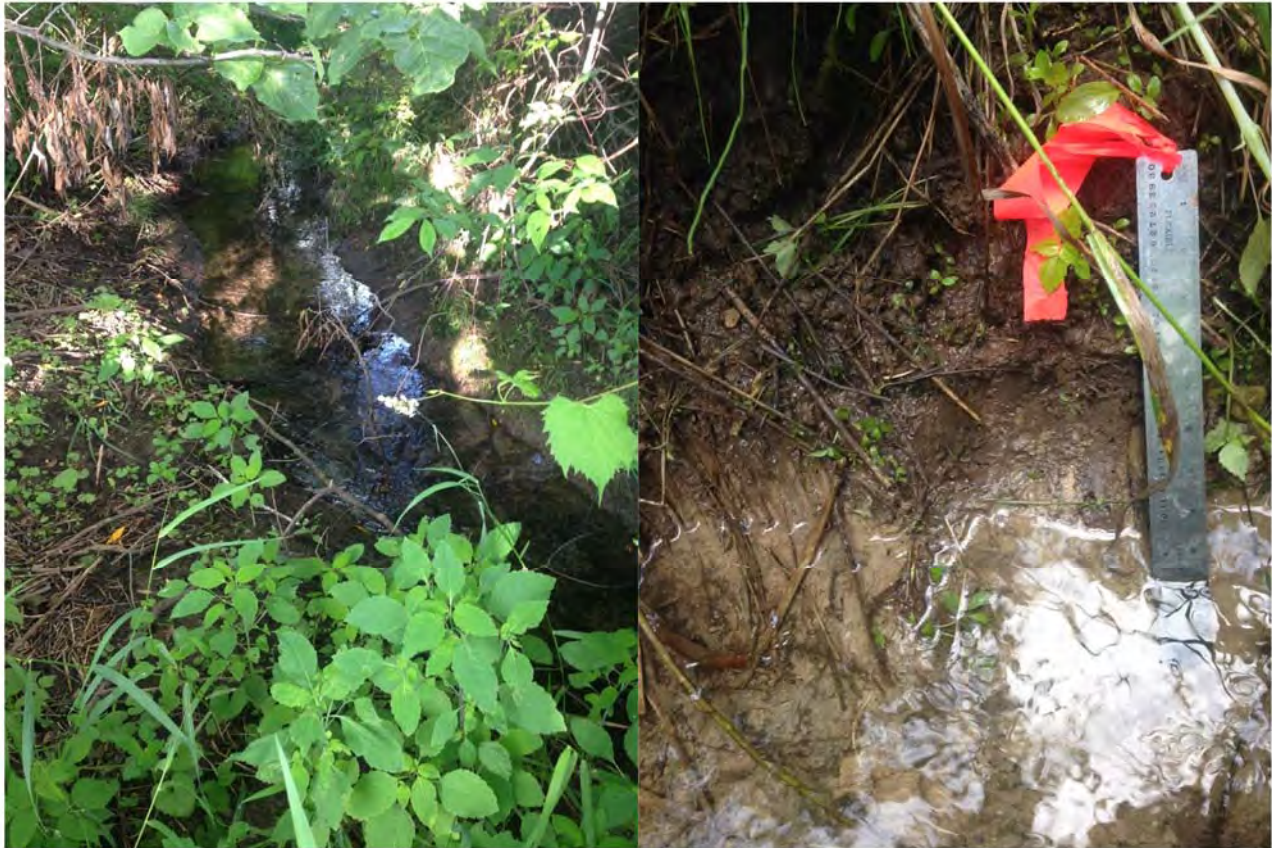
Figure 3-14 Downstream Depositional Channel With Developed Floodplain (left) and Actively Incising Upstream Reach Indicating Scour to Native Till (right)
