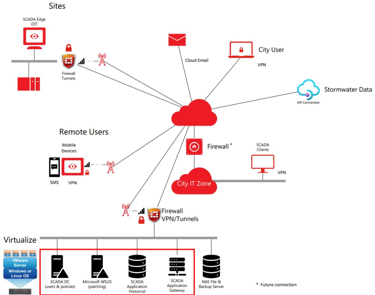
Figure 2: SCADA Architecture
