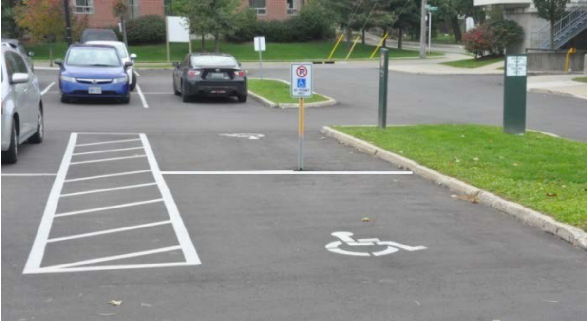
Figure 8: Example of accessible parking spaces with required signage (mounted sign and the International Symbol of Access pavement sign)
