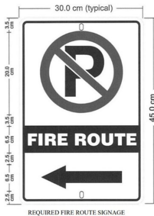
Fire Route sign
