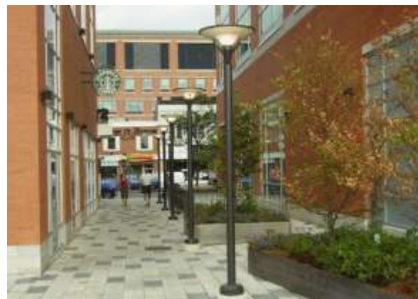
Pedestrian scale, full cut off fixtures provide safe lighting along pedestrian walkways (Waterloo).
