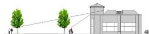
Roof top screening is evaluated through simple cross section drawings.
