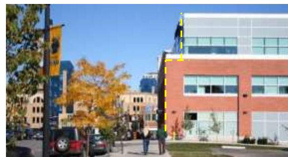
An upper storey step-back reduces the scale of building against the street (Waterloo).
