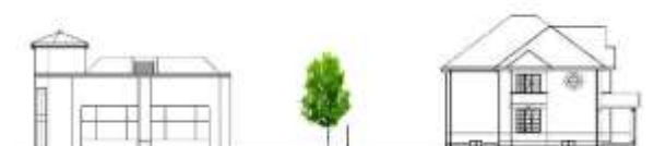
Rooftop noise is eliminated by locating rooftop equipment within a pitched roof structure.
