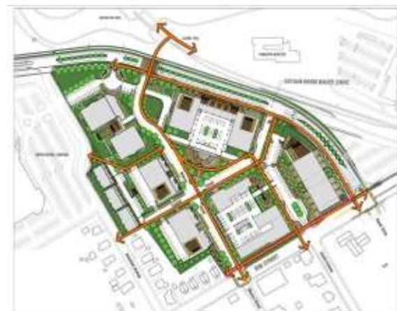
An integrated circulation system provides direct connections to surrounding streets, trails and park spaces (conceptual pedestrian circulation plan for Barrel Yards project).
