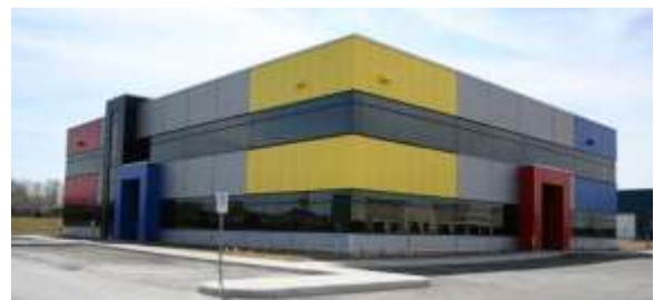
Simple building designs can be enhanced through contrasting colours, horizontal elements and projecting entrance features (Waterloo).
