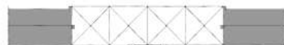
Human scale is lost when buildings are no longer able to frame the street (less than a 1:4 ratio).
