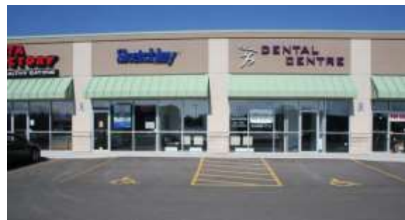
Effective accessibility is established when barrier free parking are located close to building entrances (Kitchener).
