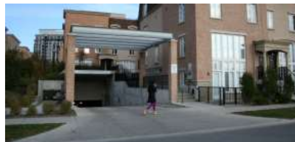
Sightlines and pedestrian safety is improved when parking garage is setback from sidewalk (Toronto).
